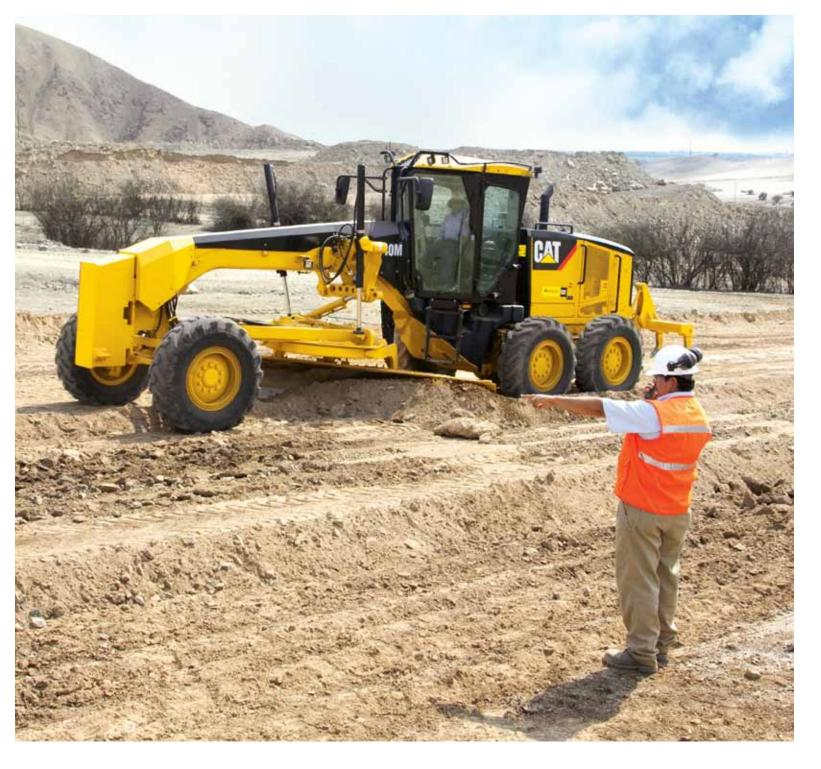
The M Series motor graders, the latest model launched by Caterpillar in this family of machines, are the leading players in an unprecedented innovation: the replacement of conventional control levers by two ergonomic joysticks that reduce the movement of hand and wrist in more than 78%. Furthermore, these machines offer exceptional visibility of the work area, among other features, configuring an alternative that provides comfort and ease of use, increasing the productivity of the operator.
